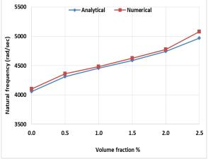
Fig. 7. Analytical and Numerical results of fundamental natural frequency for skin reinforced by SiO2 nanoparticles at mass density 1180 kg/m3
