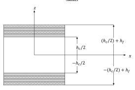
Fig. 2. Geometry of the sandwich structure layers
