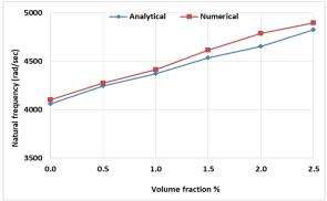
Fig. 6. Analytical and Numerical results of fundamental natural frequency for skin reinforced by Al2O3 nanoparticles at mass density 1180 kg/m3
