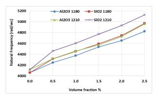
Fig. 5. The first natural frequency results of the sandwich panel at two densities for Al<sub>2</sub>O<sub>3</sub> & SiO<sub>2</sub> nanoparticles
