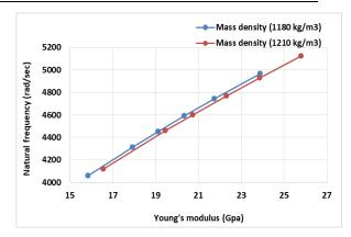
Fig. 3. The relationship of the first natural frequency with various Young's modulus of sandwich panel reinforced by SiO2 nanoparticles at two mss densities.
